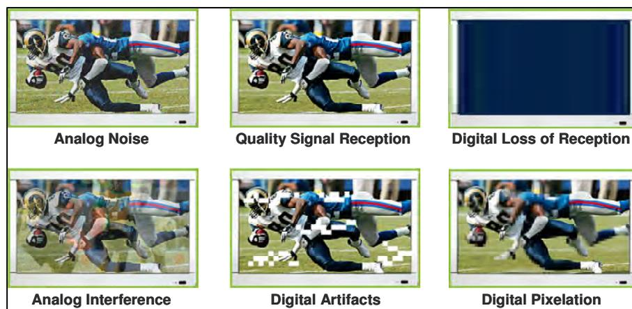
**Figure 3: High-Performance Tuners Avoid Common Reception Problems**
