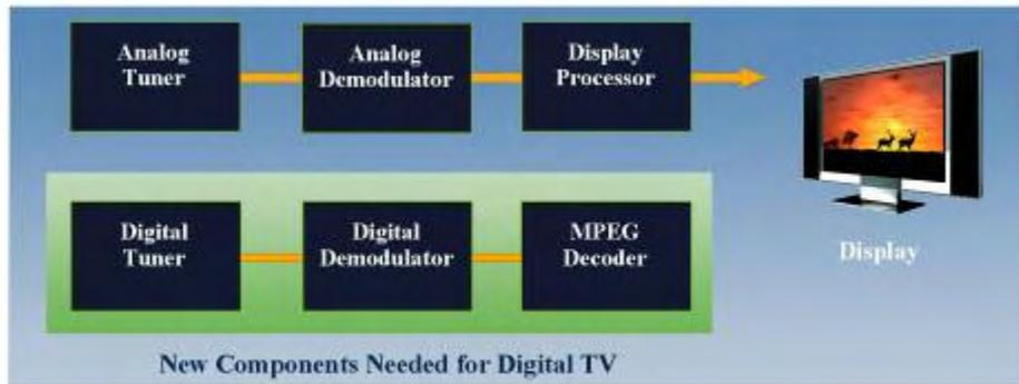
**Figure 4: TVs require a digital tuner, demodulator, and MPEG decoder to add DTV capability.**
